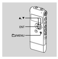
You can set the scanning sensitivity when presetting FM radio stations. The scanning sensitivity is set to "HIGH (SCAN H)" when you purchase the IC recorder.
